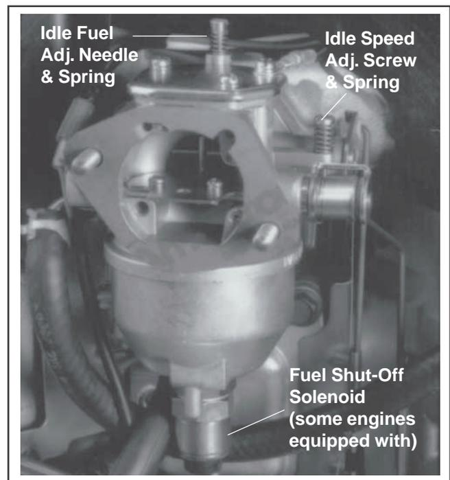
Figure 19. Carburetor CV17-25, CV675-740.
