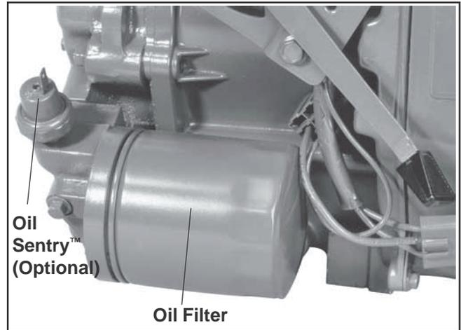
Figure 8. Oil Filter and Optional Oil Sentry™ Switch.
