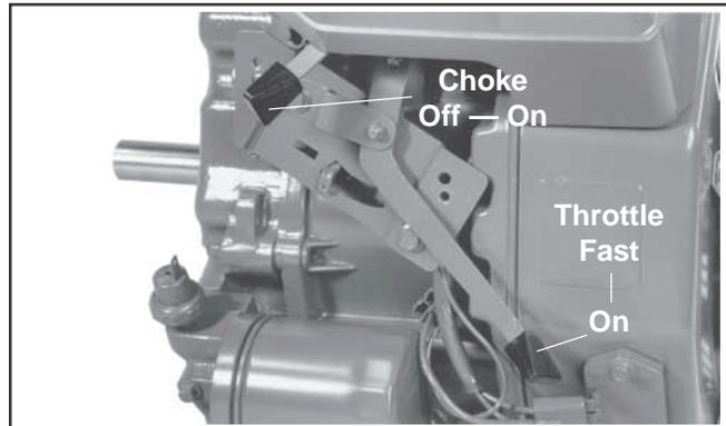
**Figure 5. Throttle and Choke Positions for Starting Engine.**
